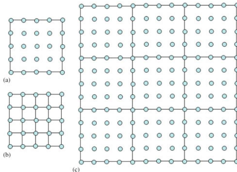
Figure 1. (a) Component substructure CS\_5  $\times$  5; (b) component substructure meshed by quadrilateral elements; and (c) quadrilateral sample domain 13  $\times$  13 nodes assembled of nine CS\_5  $\times$  5.
