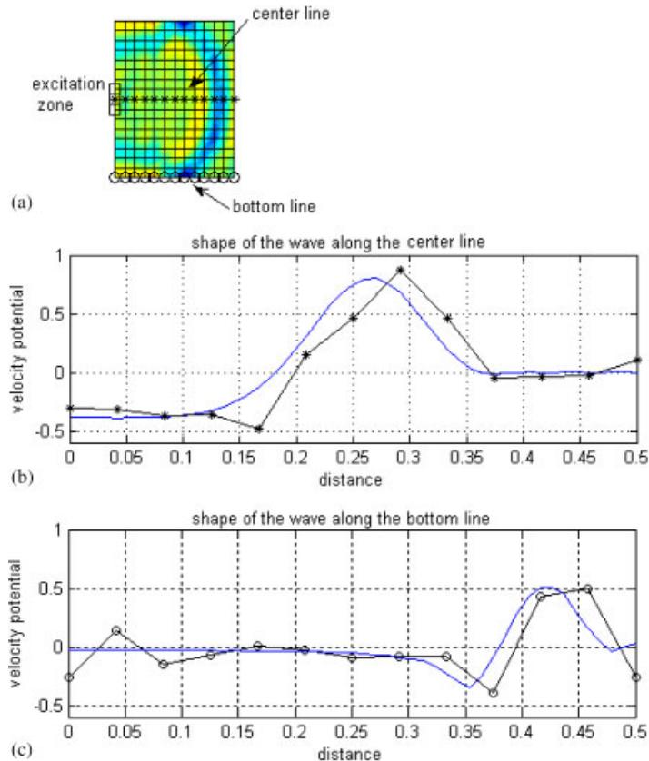
Figure 4. Acoustic wave propagating in a roughly meshed ( $13 \times 17$ ) domain: (a) rough mesh and velocity potential contour plot at a given time point; (b) reference shape of the wave (solid line) and the wave shape along the centreline of the model obtained by using the optimized CS $_5 \times 5$  (marked line-\*); and (c) reference shape of the wave (solid line) and the wave shape along the bottom line of the model obtained by using the optimized CS $_5 \times 5$  (marked line -o-).
