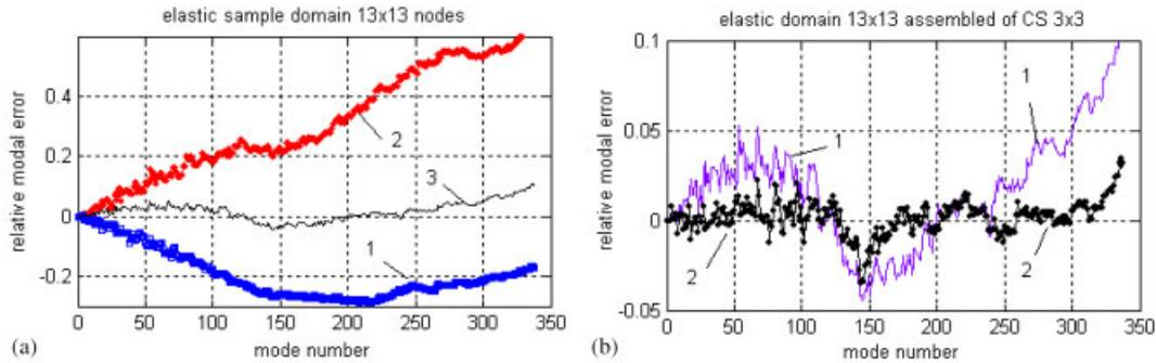
Figure 5. Relative modal errors of quadrilateral elastic sample domain  $13 \times 13$  nodes: (a) obtained by using traditional elements with lumped (1), consistent (2) and generalized (3) mass matrices; and (b) obtained by using the  $CS_3 \times 3$  optimized over 80% of modes (2) compared to quadrilateral elements with generalized mass matrices (1).
