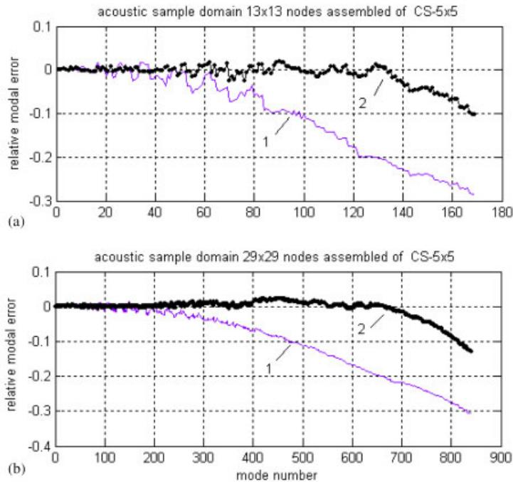
Figure 3. Relative modal errors of sample domains  $13 \times 13$  (a) and  $29 \times 29$  (b) nodes. 1—sample domain meshed by quadrilateral elements by using generalized ( $k_L = 0.35$ ) mass matrices (presented here for the sake of comparison); and 2—sample domain assembled of CS $_5 \times 5$  optimized over 80% of modes.
