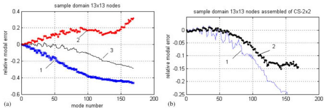
Figure 2. Relative modal errors of quadrilateral acoustic sample domain  $13 \times 13$  nodes obtained by using: (a) quadrilateral elements with lumped (1), consistent (2) and generalized  $k_L = 0.35$  (3) mass matrices; and (b) CS $_{2 \times 2}$  optimized over 30% of modes (2) compared to quadrilateral elements with generalized mass matrices (1).
